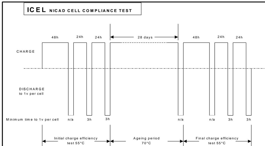
**Figure 7 - Schematic Representation of ICEL Audit Test Regime**
