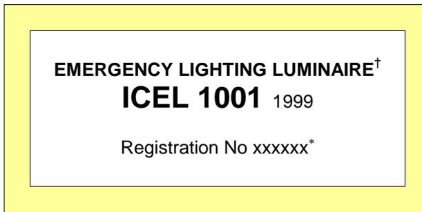
**Figure 8 - ICEL 1001 Emergency Luminaire Label Format**
